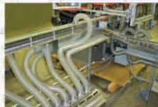
1 Stainless pneumatic conveyor: High-speed; food grade stainless steel; accommodates compact footprint.
