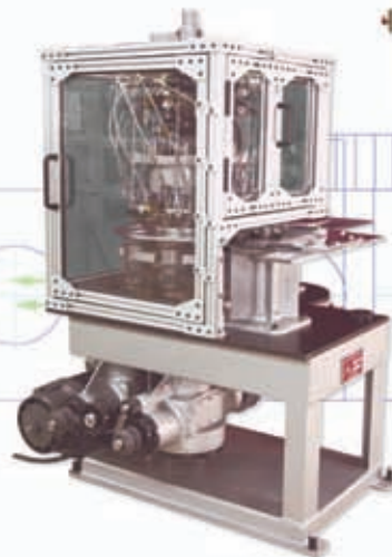
4 Apex-Swangren RCS: High-speed, smooth, continuous rotary compound pouring; 800 cpm for most sizes; electronic chuck speed and fine dispense adjustments; electronic cap presence; vacuum-capable.
